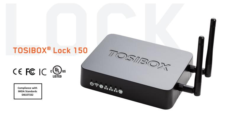
TOSIBOX® Lock 150 is an industrial router with firewall and secure Plug &  $Go^{\intercal}$  connectivity. It serves as an endpoint for secure remote connections.
