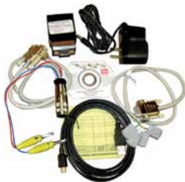
Figure 2. G-Series PC Programming Kit, part no. 253311-1
