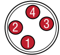
Input voltage, male, 4-pin (M8) integral connector pin-out as viewed from the end of the sensor
