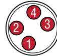
Input voltage, male, 4-pin (M8) integral connector pin-out as viewed from the end of the sensor
