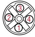
Female, 4-pin (M12-D) Integral connector pin-out as viewed from the end of the sensor
