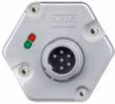
Figure 3. G-Series sensor diagnostic LEDs
