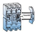
The shunt trip opens the mechanism in response to an externally applied voltage signal. The releases include coil clearing contacts that automatically clear the signal circuit when the breaker has tripped. This is not available for ELCBs of 30~250AF.
