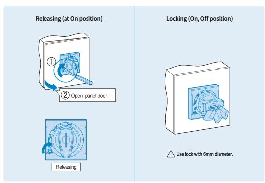
Note: In case of EH100/125/250 Semi Type, it is possible to lock E-handle only in the condition of OFF.
