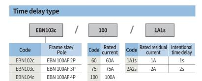
Note) EBN103c/100/30: EBN103c, Rated current 100A, Time delay type 1A1s
