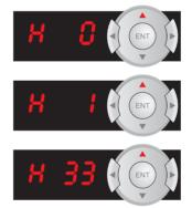
In this example, we will set Parameter H33 (Function Group 2 "H", Parameter number 33) which is motor rated current.
