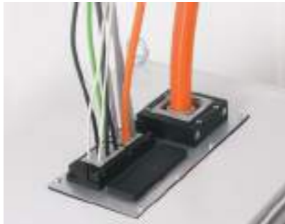
Routing of several cables with and without connectors through a closed enclosure roof via module plates. Cut-out size 314 × 144 mm.
