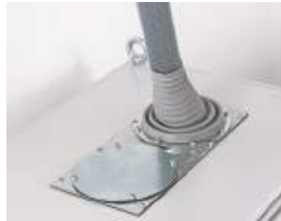
Routing of a rigid supply line through a closed enclosure roof via module plates. Cut-out size 314 × 144 mm.
