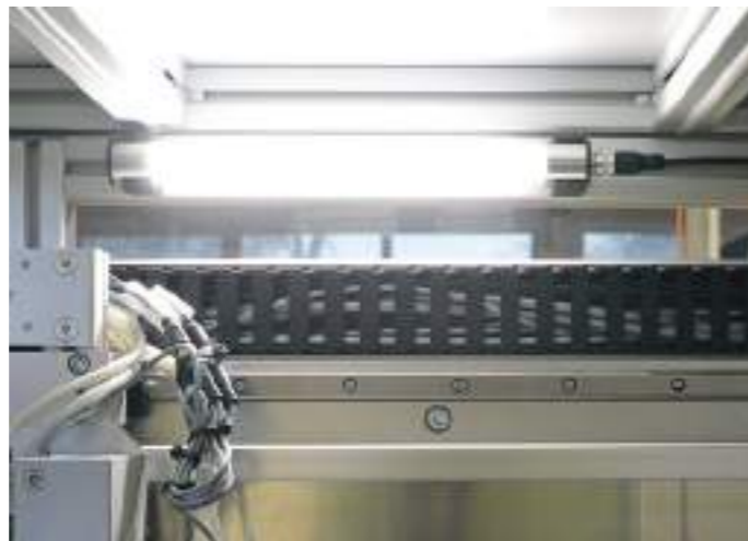
LED tube in polycarbonate
