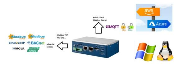
Using a PC as the gateway provides exceptional flexibility, enabling customized solutions. Our setup runs on Linux OS with Node-RED for software, but it's also compatible with Windows.
